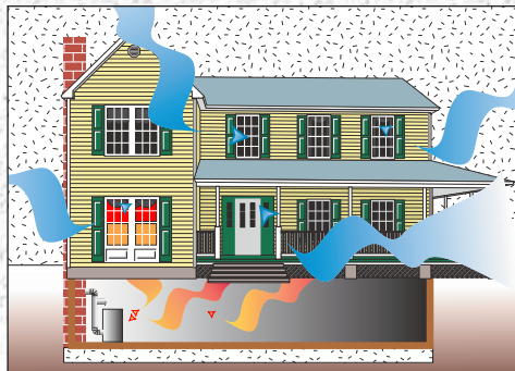
Ordinary boilers consume warm household air which causes infiltration of chilly outdoor air to replace it.
